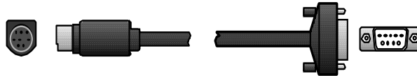
Macintosh Modem Port (8-pin DIN) to Edit Suite's Computer (RS-232C) DB-9 Port
